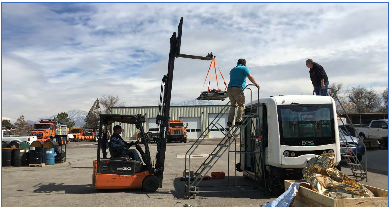
Assembling the roof-mounted HVAC and sensor unit atop the shuttle
